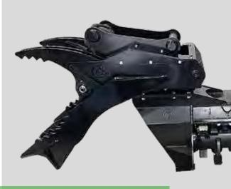
Support foot with integrated grapple: Reinforced stability and easy handling, even on uneven terrain.
